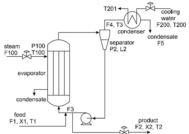
Fig. 3. Evaporator system
