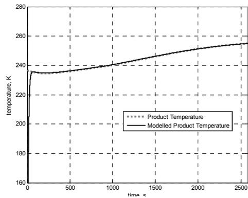
Fig.4. Modeling of relation in a Lyophilization cycle
