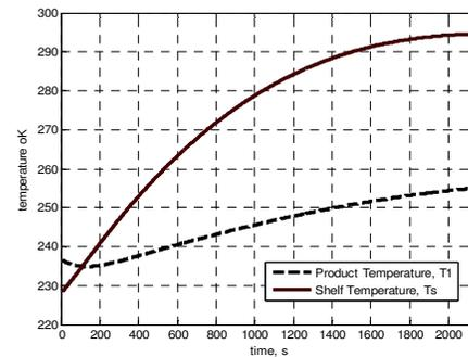
Fig.7. Product and Shelf temperatures in case of Model Predictive Control scheme with FNWH model at  $\rho=0.0003$ .
