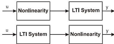
Fig.1. Structures of classical Hammerstein and Wiener models
