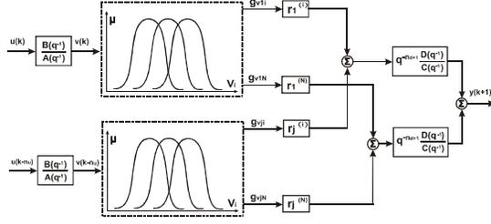
Fig.3. Fuzzy-Neural Wiener-Hammerstein model
