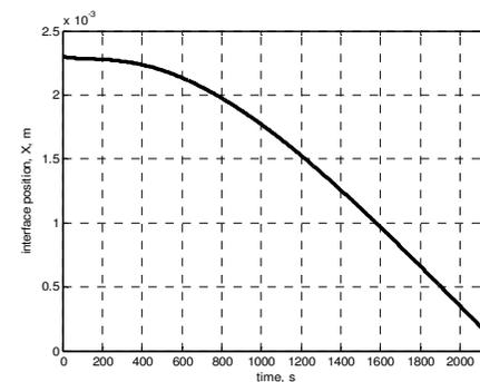
Fig.8. Interface position during the drying process in case of Model predictive control scheme with FNWH model at  $\rho=0.0003$ .
