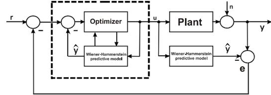
Fig.4. Block diagram of the proposed model predictive control system
