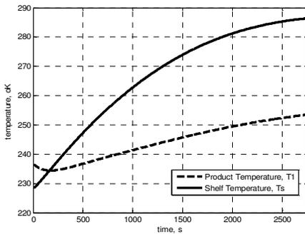
Fig.9. Product and Shelf temperatures in case of Model Predictive Control scheme with FNWH model at  $\rho=0.00022$ .
