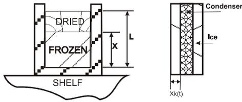
Fig.6. Schematic diagram of sublimation in a vial and condensation of the evaporated water at the condenser.
