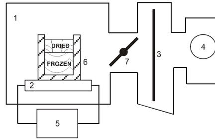
Fig.5. Schematic diagram of a simplified Lyophilization plant.
