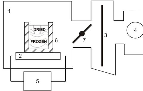
Fig.5. Diagram of simplified Lyophilization plant
