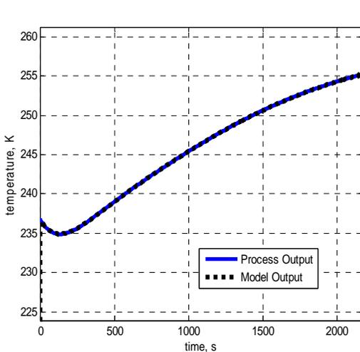
Fig.6. Process and Model outputs during a Lyophilization cycle
