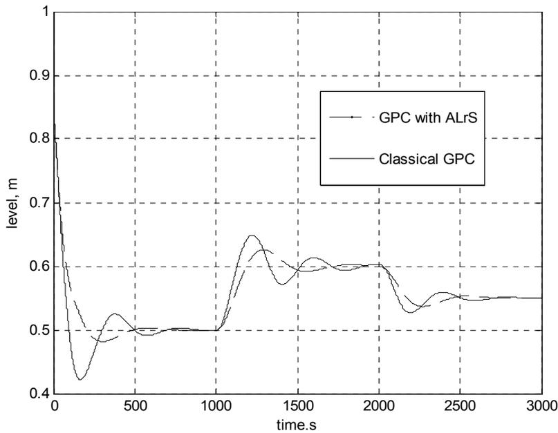
**Fig. 6** Transient process responses in case of variable reference and  $\rho=0.0015$
