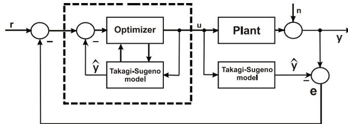
**Fig. 1.** Block diagram of model predictive control system
