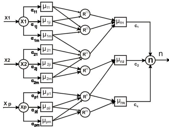
Fig. 2. The structure of the proposed ALrS neural network
