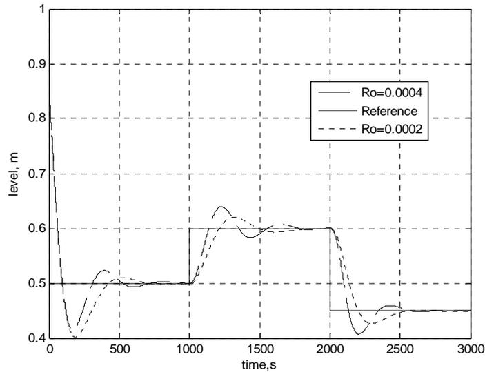
**Fig. 6.** GPC using Fuzzy-Neural Hammerstein model at different values of  $\rho$
