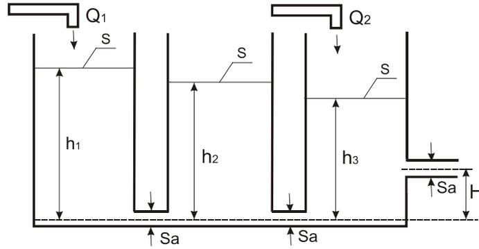
Fig. 4. The model of the three cascaded water tanks
