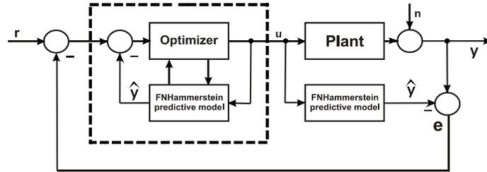
Fig. 3. Block diagram of model predictive control system
