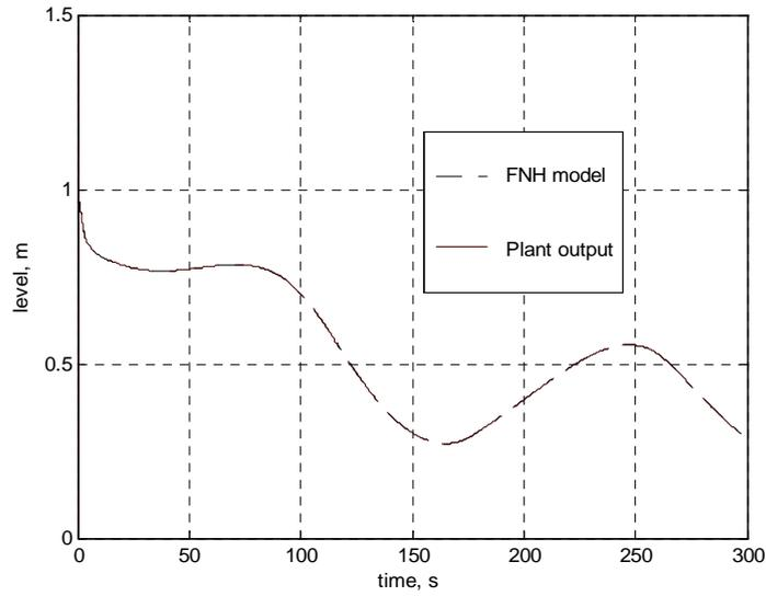
**Fig. 5.** Training of the FN-Hammerstein model with sinusoidal signal
