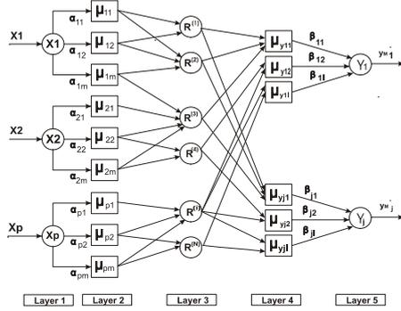
Fig. 1 The structure of the proposed fuzzy-neural network
