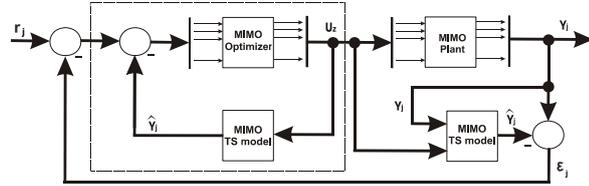
Fig.2 Block diagram of MIMO model predictive control system
