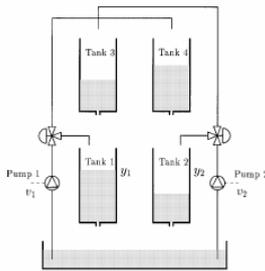
Fig.3 The quadruple-tank process
